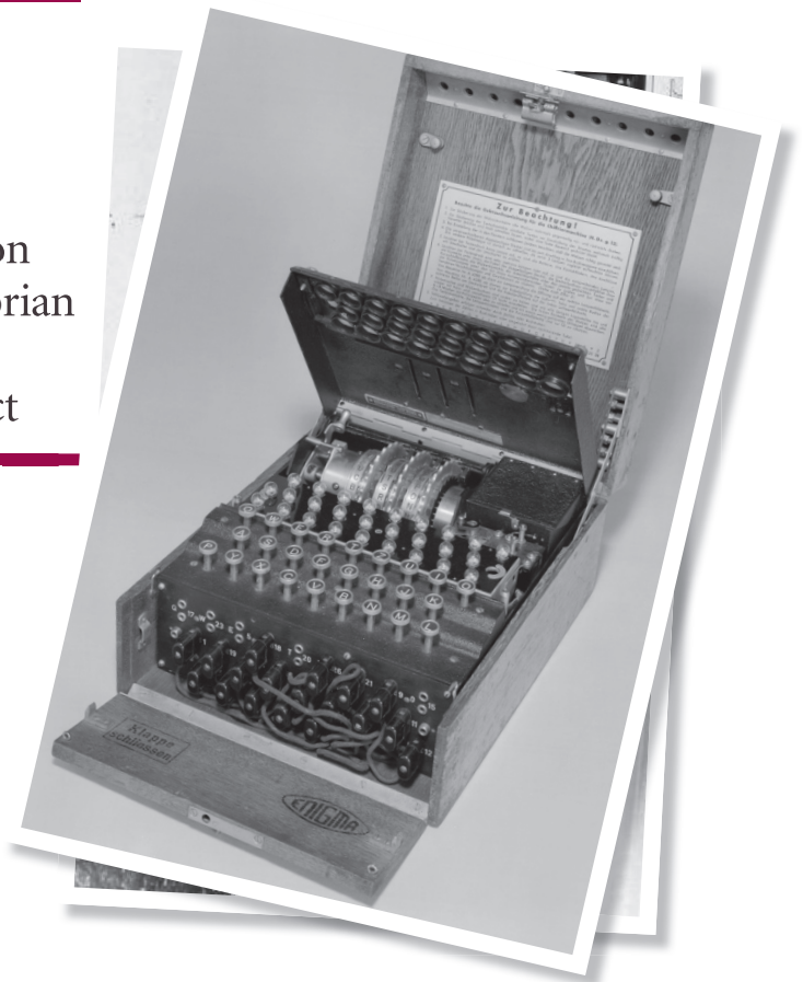
An Enigma cipher machine, used by Germany during the Second World War to keep its communications secret. The machine's rotors created billions of combinations of letters to scramble messages. The Germans believed in the absolute security of the Enigma, but with the help of Polish mathematicians, British codebreakers cracked the code. The intelligence gathered by intercepting coded messages – and keeping secret the fact that the German code system had been broken – was vital to winning the war. These events were kept secret until 1974. Photograph: Getty Images
